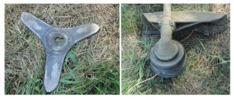
Figure 1. The employed cutting heads used during trials: brush knife (left) and mowing head (right)
