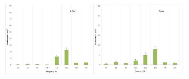
Figure 3. Input spectra in one-third octave band calculated as the average (±s.d.) of the six operators (left: brush knife; right: mowing head)
